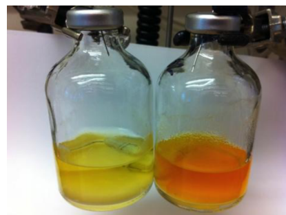
Figure 2. Color change indicating completion of borylation reaction: (left) completion of borylation on an aryl chloride; (right) completion of borylation of an aryl bromide.
